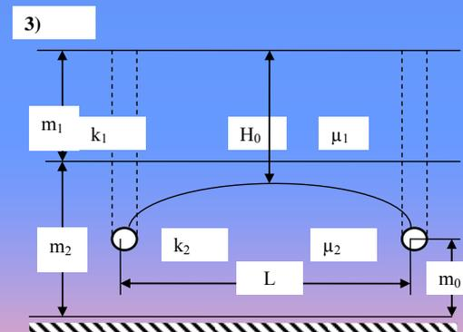
Pic.2. Calculation schemes for systematic drainage system design.
